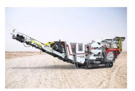
The E-Series Electric-Driven Mobile Crusher
