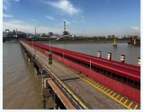
The dust hood of the belt conveyor can suppress dust and control noise
